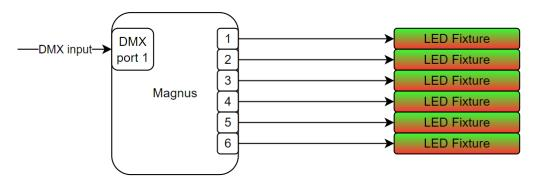
The DMX input is set to mode "slave", and setup to trigger start/pause/stop on player 1. The file in player 1 was preloaded.
