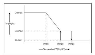
The values are configured in the MaNima Configurator. The lower end features an hysteresis, to make sure the LED fixture wont start blinking on this edge case.
