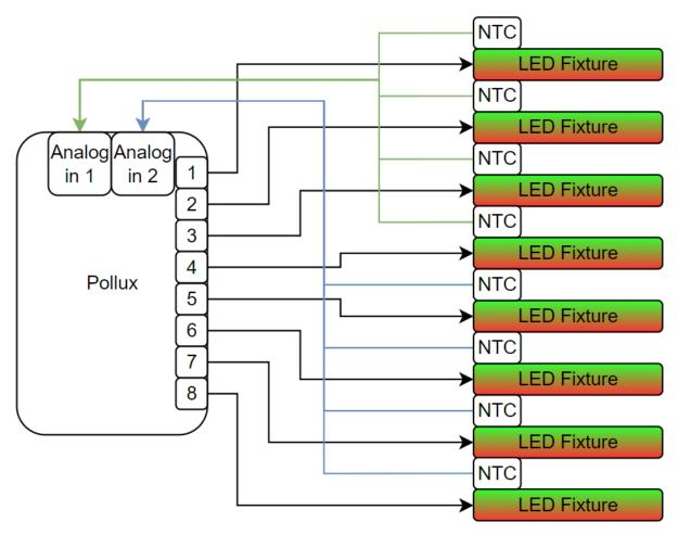
In this case, each fixture contains its own NTC. In practice, this is often not required, as the measured temperature will be about the same if equal type of fixtures are used.
