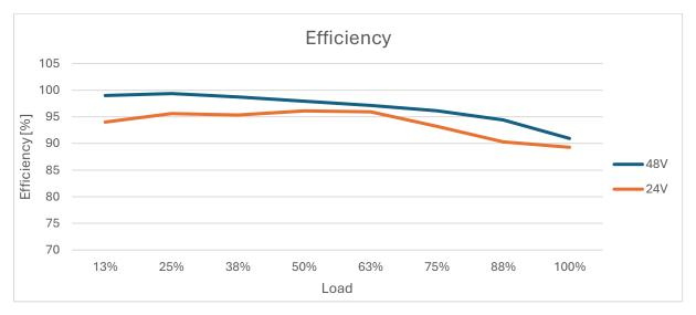
100% load means 2000W of output power driven with 100% duty cycle.
